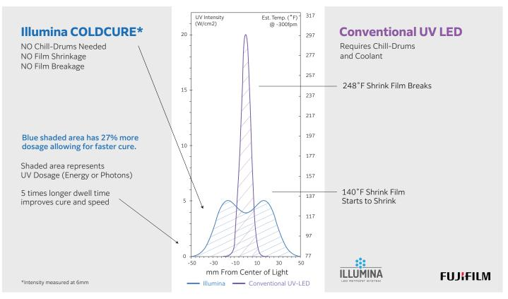
As illustrated in the chart above, the UV dosage of the Illumina COLDCURE process is below the 140°F indicator line where shrink film begins to shrink, so heat and its effects are taken out of the equation. The COLDCURE benefits of Ultra Low Temperature plus High Dosage and Dwell Time are numerous.
