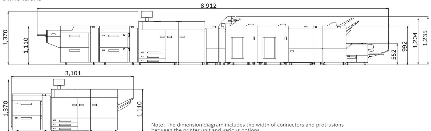
Note: The dimension diagram includes the width of connectors and protrusions between the printer unit and various options.
