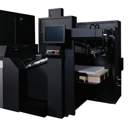
All of this translates into higher quality, shorter runs, and more cost-effective jobs than traditional offset platforms. Built on a traditional offset press frame, the J Press 750 handles sheets the same as an offset press, prints on standard offset stocks and finishes like an offset sheet.
